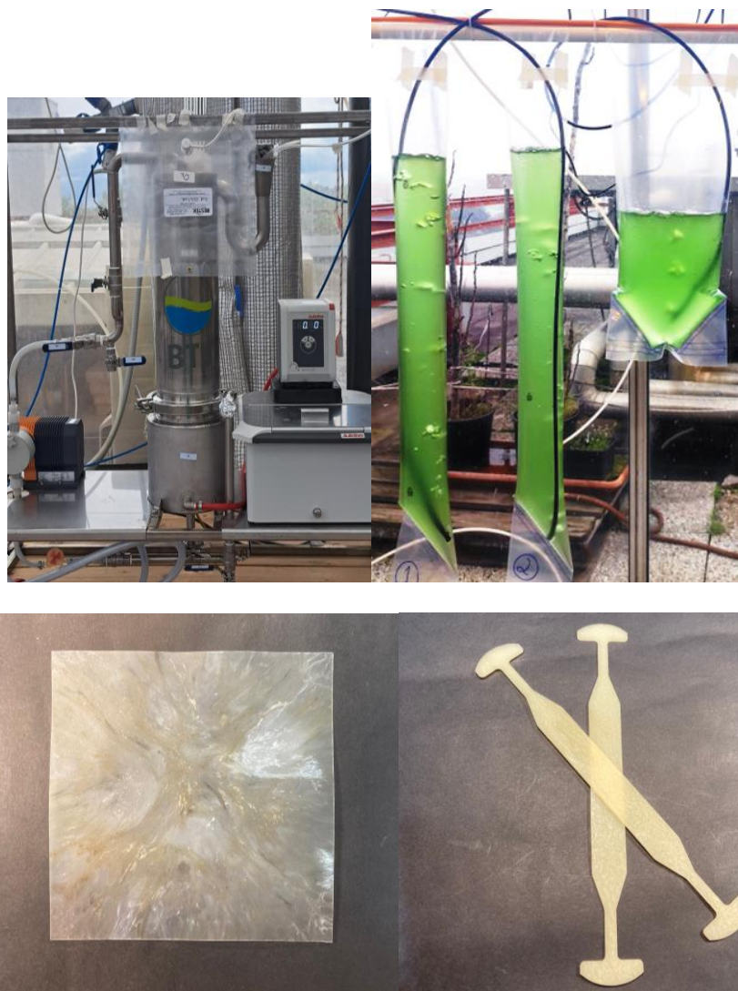
Figure 2. Bioreactors and photobioreactors used for PHB production with C. necator (top left) and Synechocystis sp. B12 (top right). Samples of PHB produced at UniPD have been tested as laminates (bottom left) and packaging applications are being developed (bottom right).
