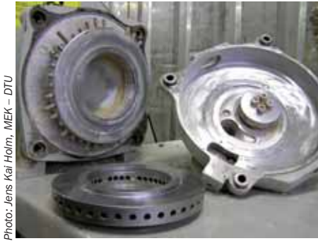
Rotating pellets press taken apart for inspection purposes.
