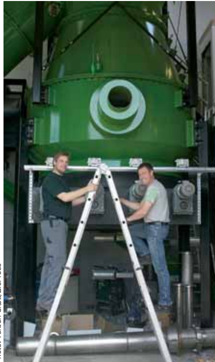
The tar-free wood chip vaporizer constitutes "the heart" of the new plant. Mads Nielsen from TK Energi (left) and production manager Torben Brand Andersen (right).
