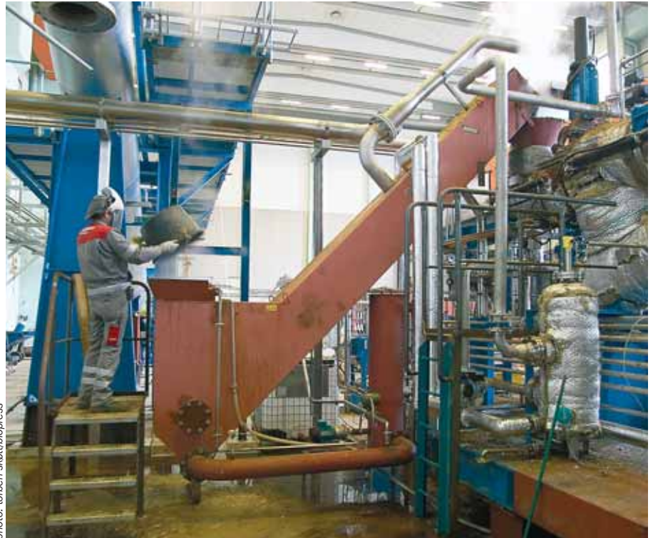
At Skærbæk power station at Fredericia, DONG Energy is far ahead with the development of a technology that makes it possible to extract ethanol from straw and use the residual product as fuel.
