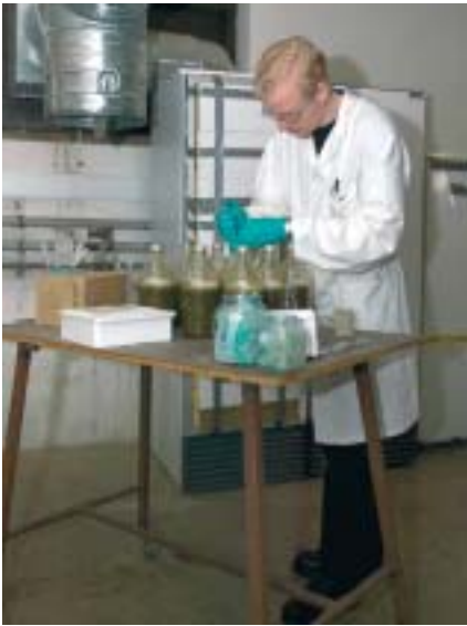
Student Verner Holm carries out tests where enzymes are added to increase the gas production.
