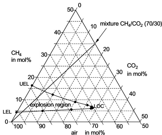
Fig. 4. Explosion region of methane-carbon dioxide-air mixture (acc. to DIN 51649, 20 °C, atmospheric pressure).
