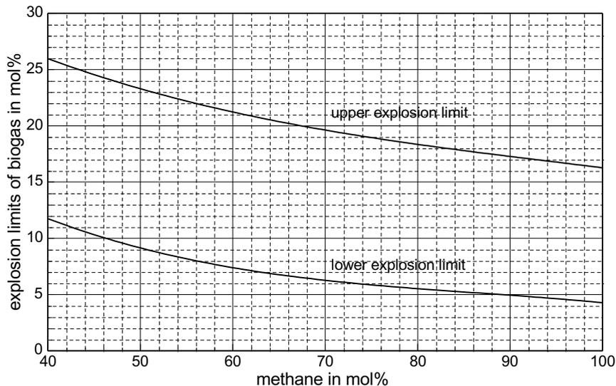
Fig. 6. Explosion limits of biogas at known methane content.
