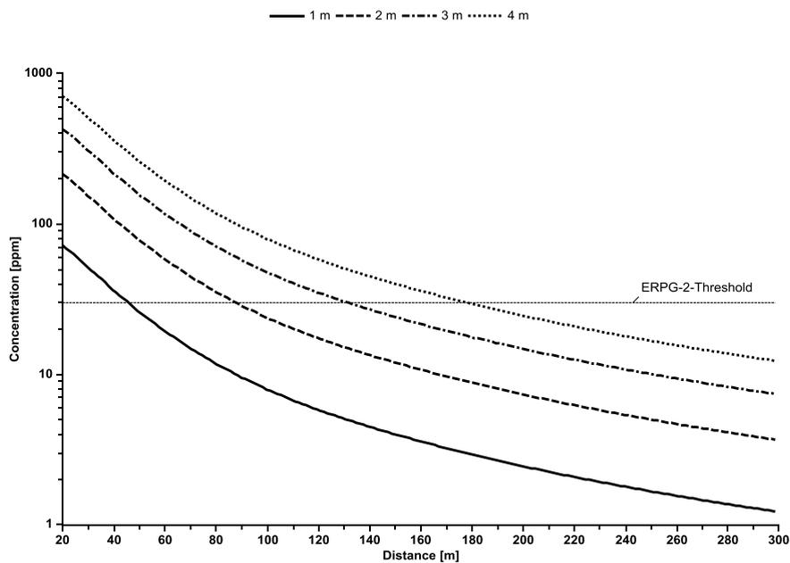
Fig. 10. Concentration of H<sub>2</sub>S against distance for different lengths of cracks.
