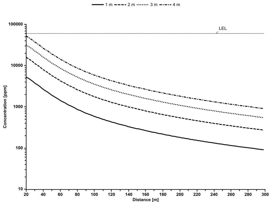
Fig. 11. Concentration of biogas against distance for different lengths of cracks.
