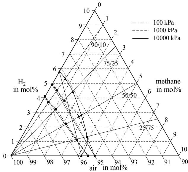
Fig. 8. Lower explosion limits of hydrogen-methane mixtures at 20 °C and pressures of 100, 1000 and 10000 kPa.
