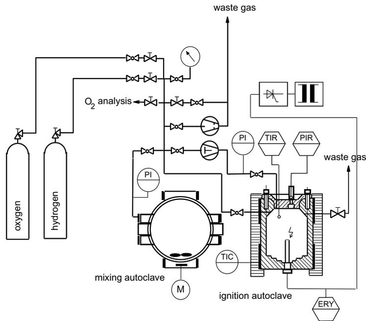
Fig.3. BAM apparatus according to EN 1839 "Bomb method".
