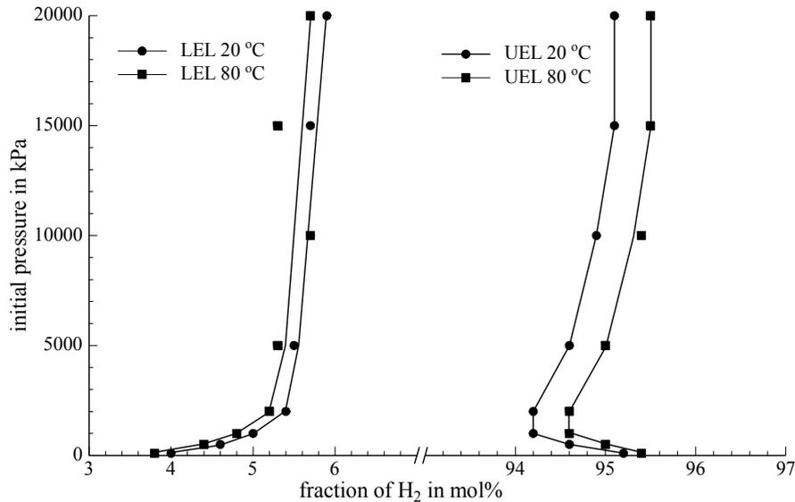
Fig. 7. Explosion limits of hydrogen in oxygen at different initial pressures
