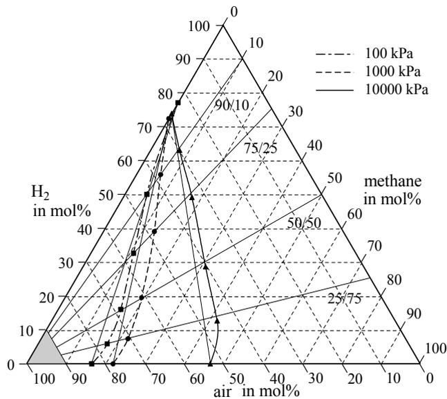
Fig. 9. Upper explosion limits of hydrogen-methane mixtures at 20 °C and pressures of 100, 1000 and 10000 kPa.
