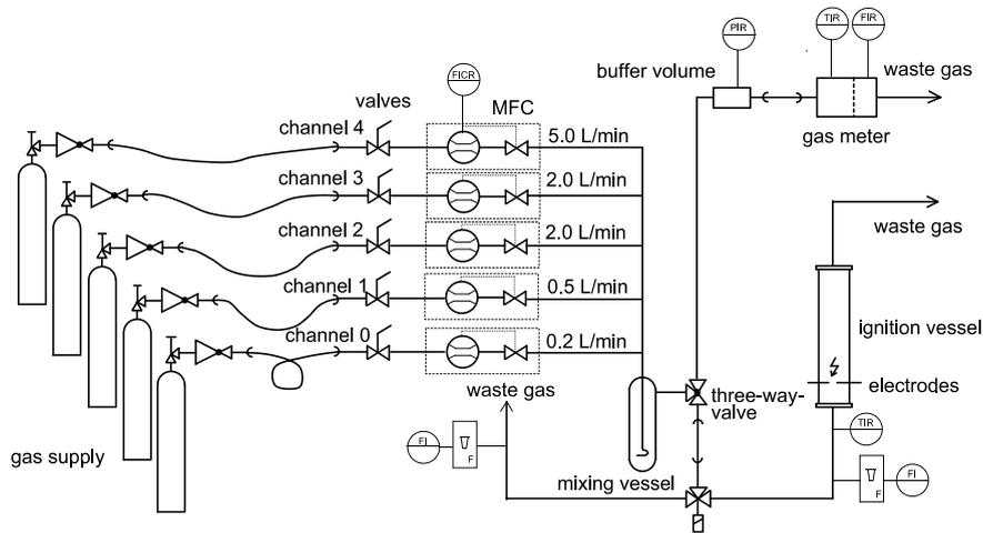
Fig. 2. BAM apparatus according to DIN 51649 and EN 1839 “Tube method”.
